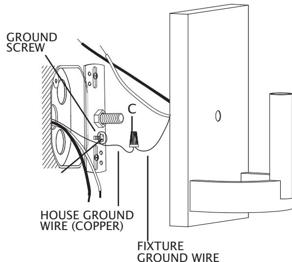
6. Twist end of house lead wire (black) and end of fixture lead wire together. Twist wire nut (C) onto ends of wires. Completely tighten wire nut (C). Twist end of house neutral wire (white) and end of fixture neutral wire together. Twist wire nut (C) onto ends of wires. Completely tighten wire nut (C). Reference chart to the right for correct wire connections.
