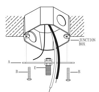
**IMPORTANT**: The length of the cord must be adjusted before fixture is installed.
